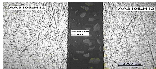
Figure 5: Microscopic bonded joint after using emery paper (ASTM 1000) of group (Al-Al-Al).
