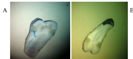
Figure 1: (A) dye penetration for group 1: Nano ceramic composite, (B) group 2 Nano ceramic composite with using surface sealant.
